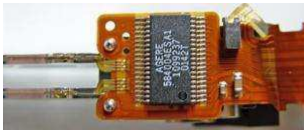
Figure 2 — a frame-type preamplifier (Seagate Barracuda IV drive)
