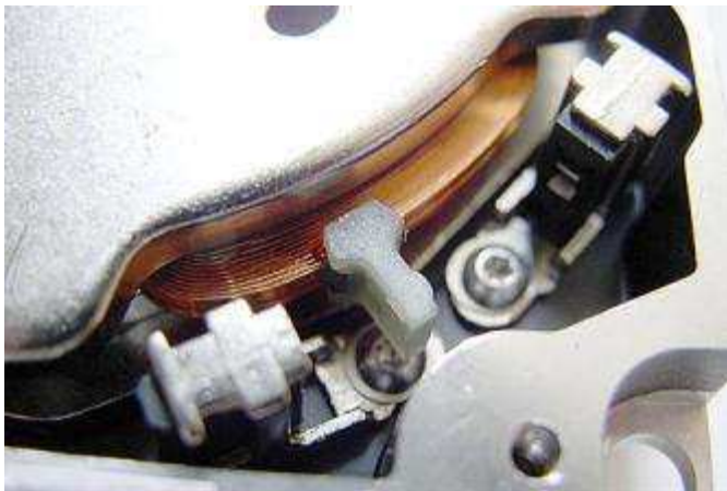
Figure 11 —ST3660A— plastic limiter
