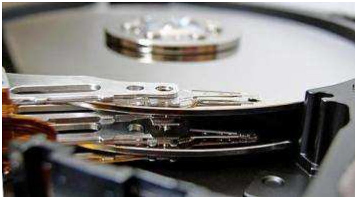
Figure 22 — A head stack (WD600BB) — heads number 0, 1 and 3 are physically present; head number 2 is missed
