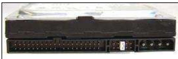
Figure 2: Connectors ATA interface.
