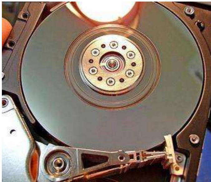
Figure 15 — Surface damage caused by a damaged head
