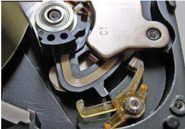
Figure 20 — A load/unload system with a magneto-mechanical principle (WD200EB)
