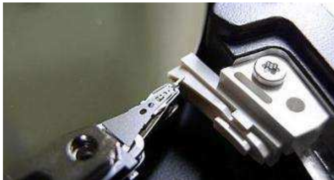
Figure 13 — Heads are loaded onto the surface (Hitachi AVV2 series hard drive, 80 GB)
