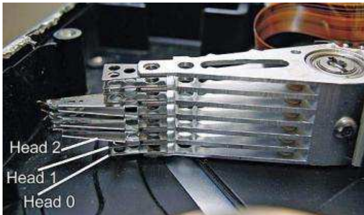
Figure 21— A heads numbering scheme (SCSI Western Digital)
