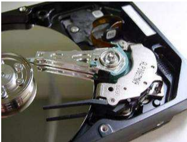
Figure 9 —plastic airlock visible
