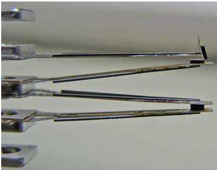
Figure 3 — "lifted" head of the 406 MB Quantum Pro Drive LPS
