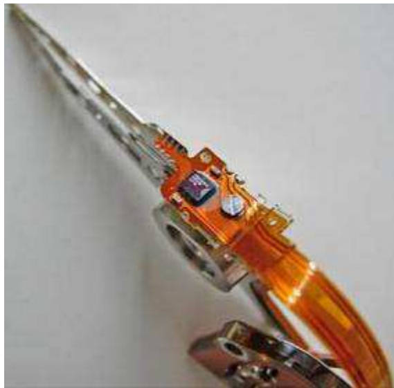
Figure 1 — a head stack with an open-frame preamplifier (Hitachi ATMR series, 2.5-inch drive)
