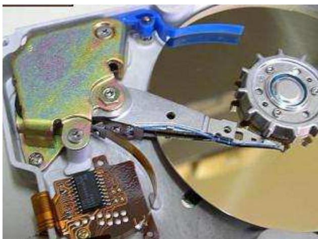
Figures 16, 17 — A load/unload system of Quantum HDD. Figure 16 — Quantum Maverick.
