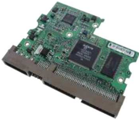
Figure 4: Logic board ATA hard drive.
