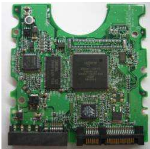
Figure 5: Logic board SATA hard drive.
