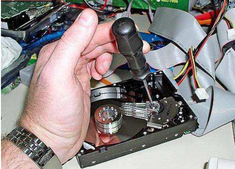
Figure 23 — after heads had been replaced, author would have to adjust manually a gradient angle of a head stack axis in WD200BB hard drive to get data
